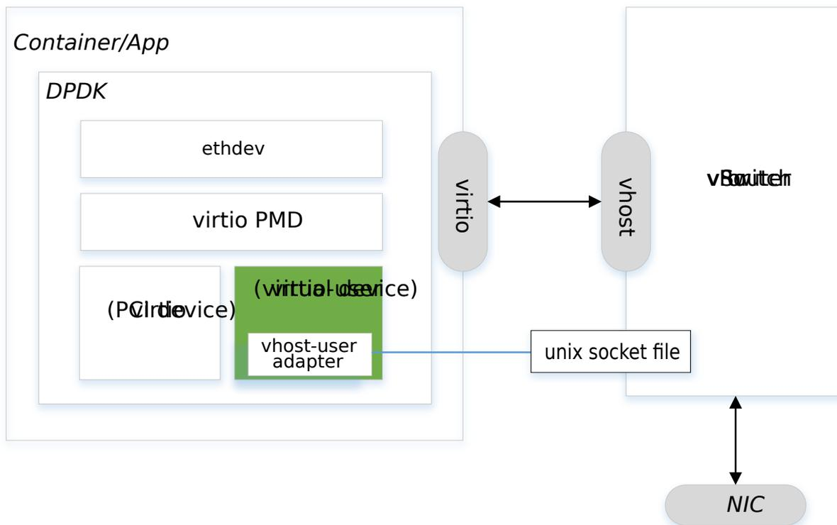
Fig. 6.2: Overview of accelerating container networking by virtio-user
