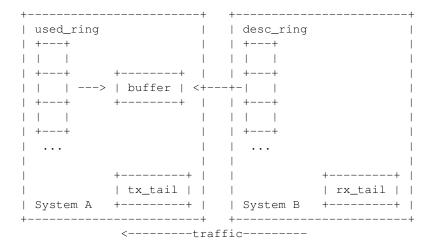
• Enqueue and Dequeue Based on this ring layout, enqueue reads rx\_tail to get how many free buffers and writes used\_ring and tx\_tail to tell the peer which buffers are filled with data. And dequeue reads tx\_tail to get how many packets are arrived, and writes desc\_ring and rx\_tail to tell the peer about the new allocated buffers. So in this way, only remote write happens and remote read can be avoid to get better performance.
