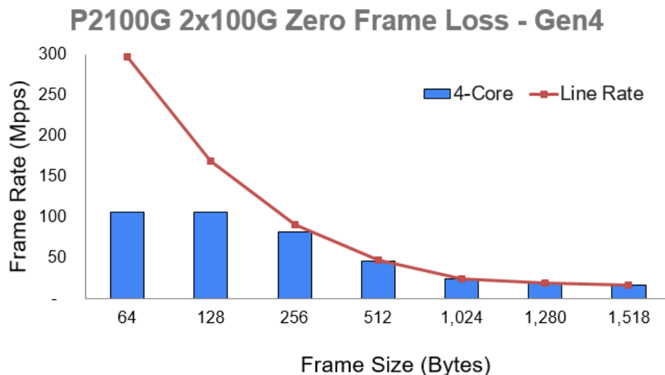
Figure 12: Results of P2100G 2x 100G Zero Frame Loss Test – PCIe 4.0
