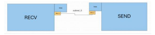
A Sender VM sends traffic to a Receiver VM using dpdk-testpmd. The Sender VM sets the testpmd -tx-ip flag to the destination address. Packet size is left as the default (64 bytes, UDP).
