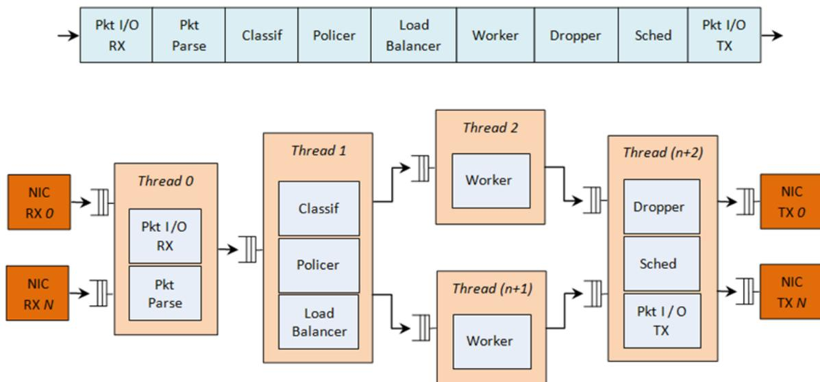
Fig. 23.1: Complex Packet Processing Pipeline with QoS Support
