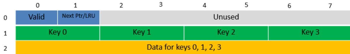
Fig. 26.6: Data Structures for 16-byte Key Hash Tables
