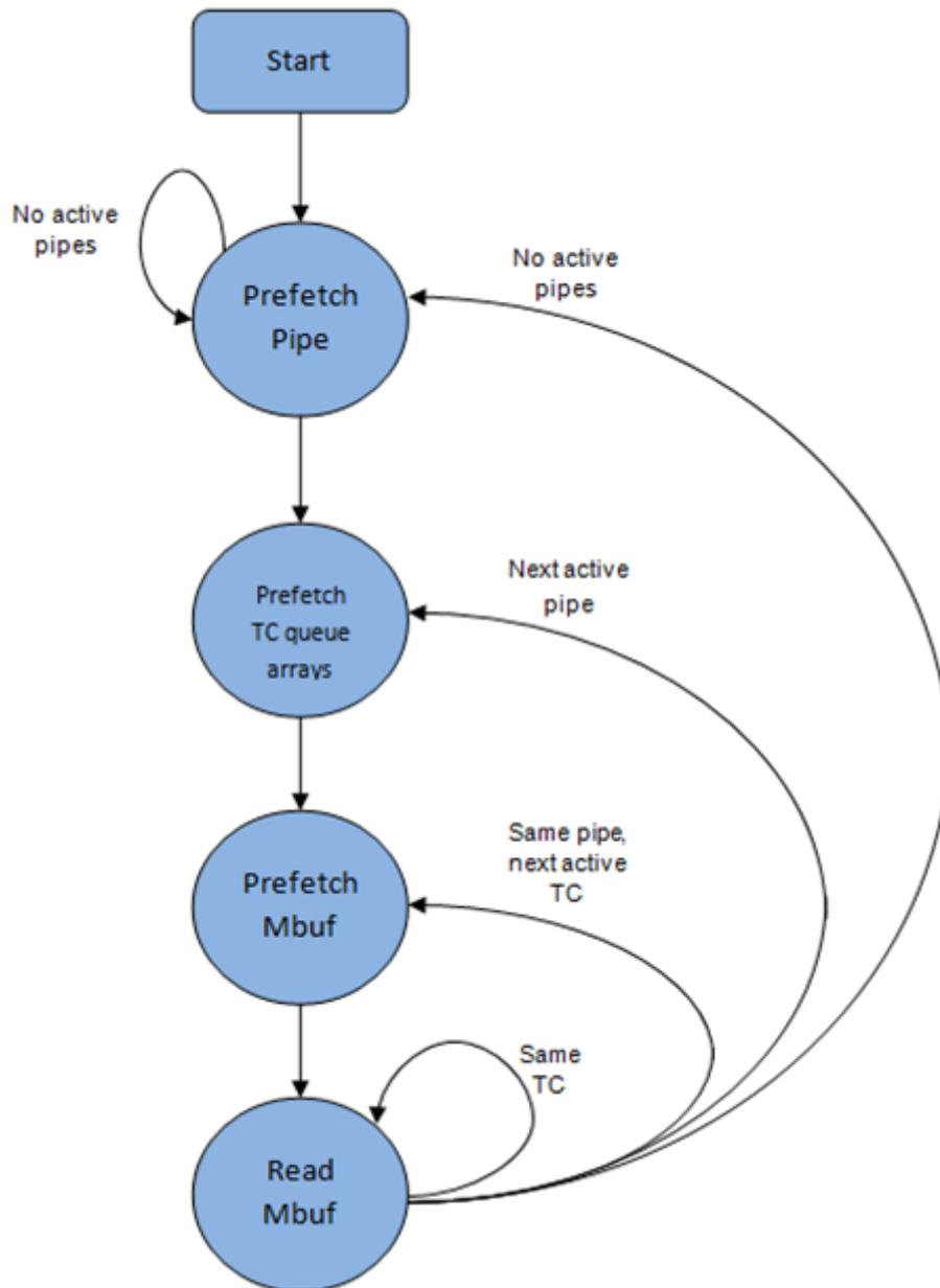
Fig. 23.6: Pipe Prefetch State Machine for the Hierarchical Scheduler Dequeue Operation
