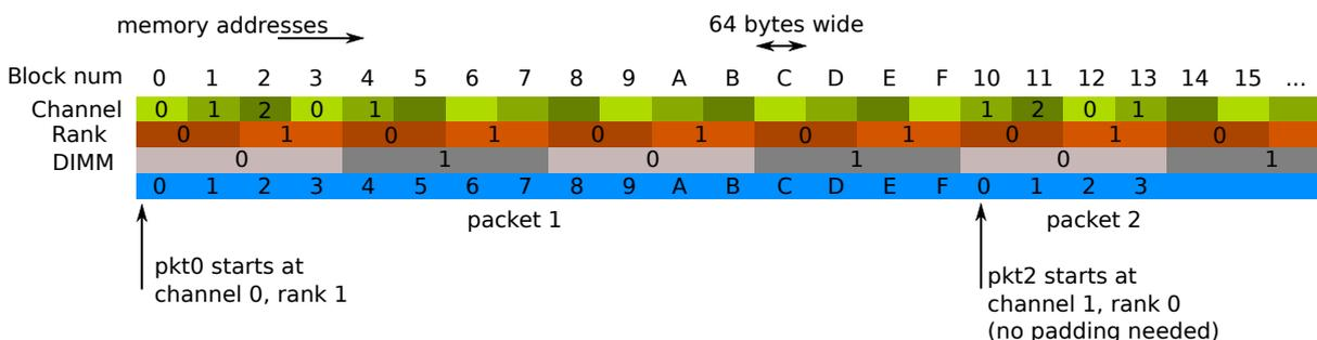
Fig. 5.2: Three Channels and Two Dual-ranked DIMM Example
