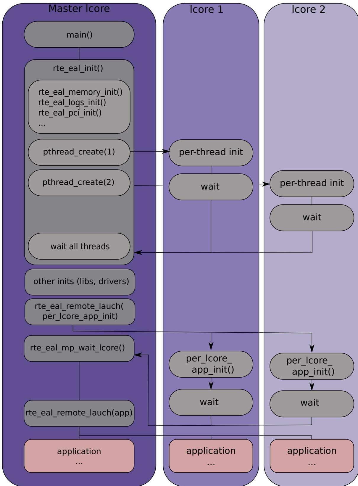
Fig. 3.1: EAL Initialization in a Linux Application Environment
