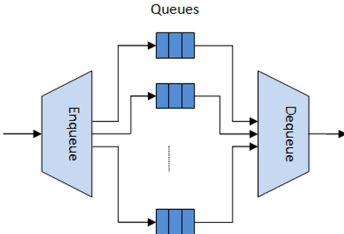
Fig. 23.2: Hierarchical Scheduler Block Internal Diagram
