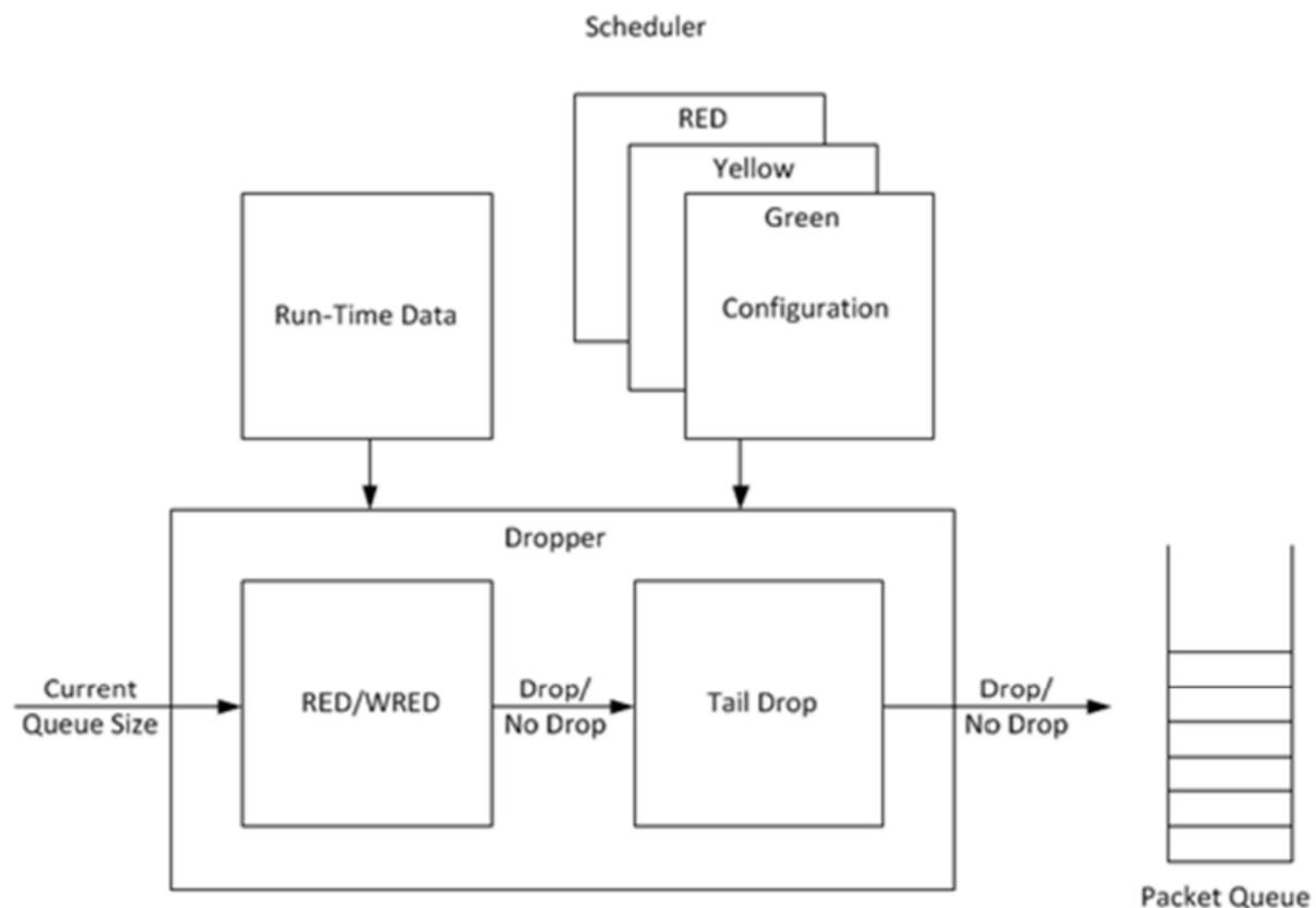
Fig. 23.7: High-level Block Diagram of the DPDK Dropper
