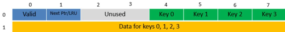
Fig. 26.5: Data Structures for 8-byte Key Hash Tables
