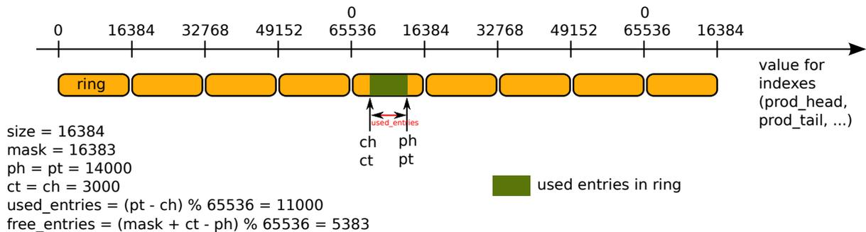
Fig. 4.13: Modulo 32-bit indexes - Example 1
