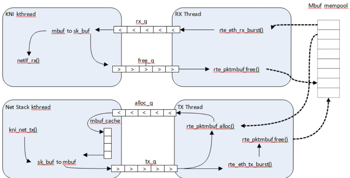
Fig. 21.2: Packet Flow via mbufs in the DPDK KNI
