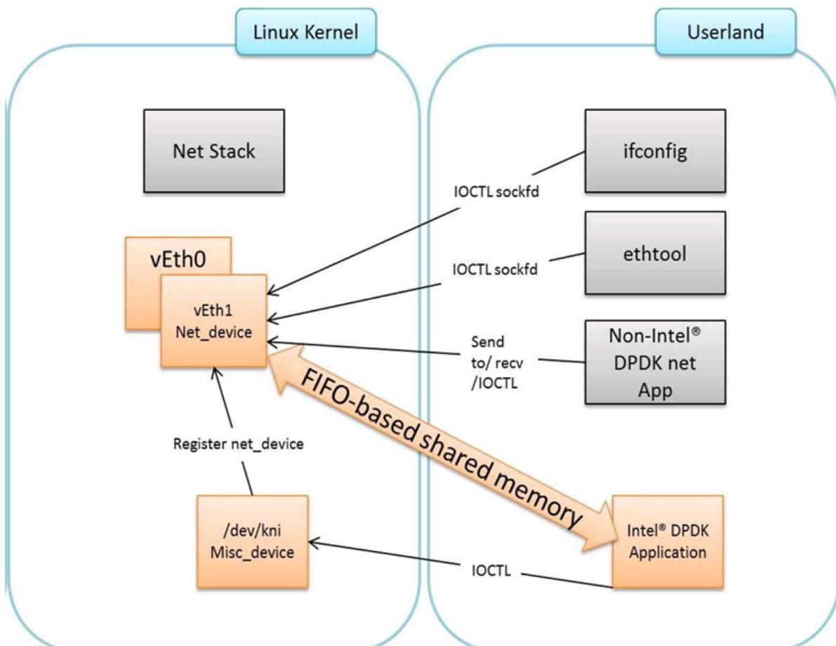
Fig. 21.1: Components of a DPDK KNI Application
