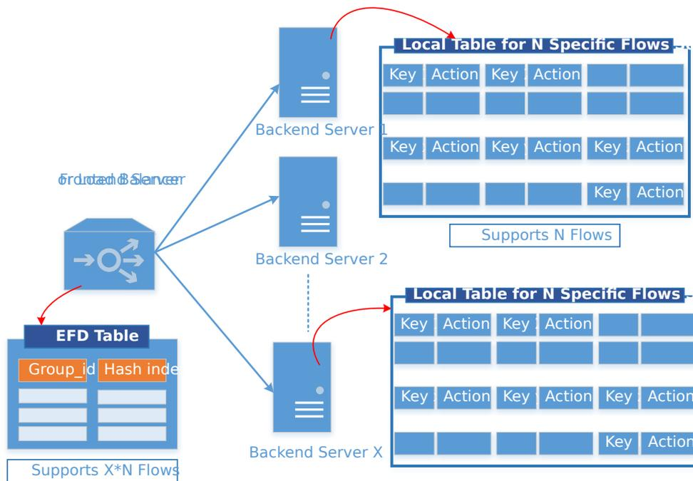
Fig. 13.6: EFD as a Flow-Level Load Balancer
