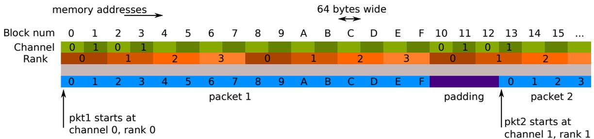
Fig. 5.1: Two Channels and Quad-ranked DIMM Example
